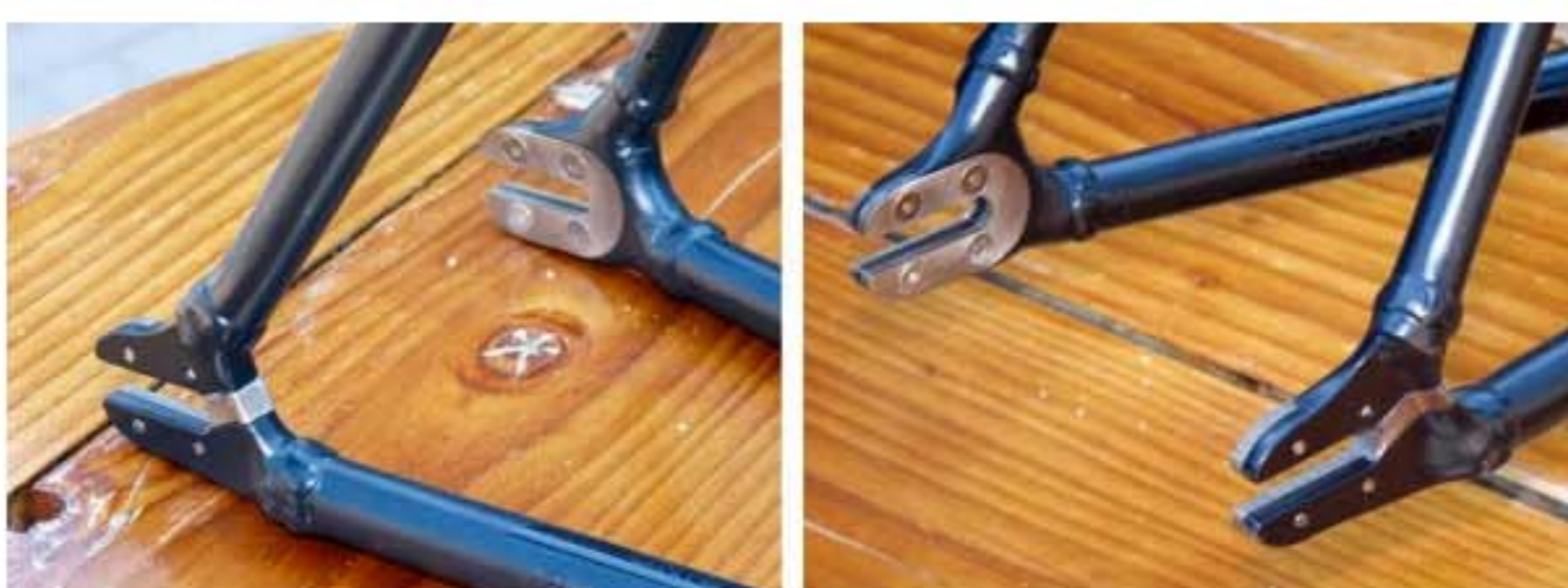
...new sliding dropouts that allow the driveside to open up for belt drive insertion. The 'cross bikes are being released first, with the Talus available by early 2012.
